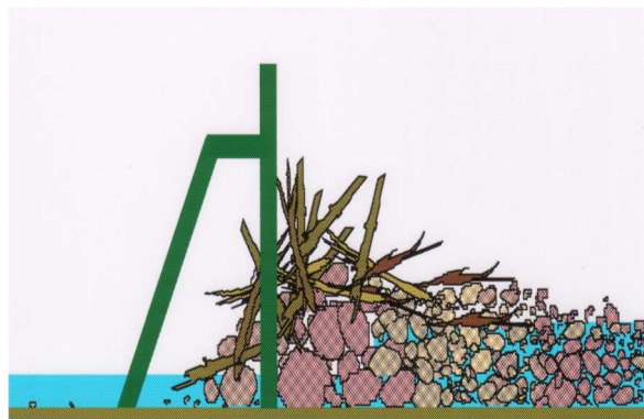
Image of a hydraulically consecutive steel frame entrapper in the bedload-flow-dominant stream section.
