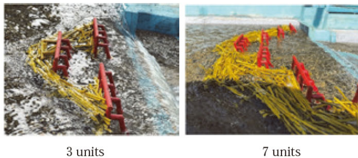
Fig. 17 Driftwood entrapment condition by the difference in number of unit components
